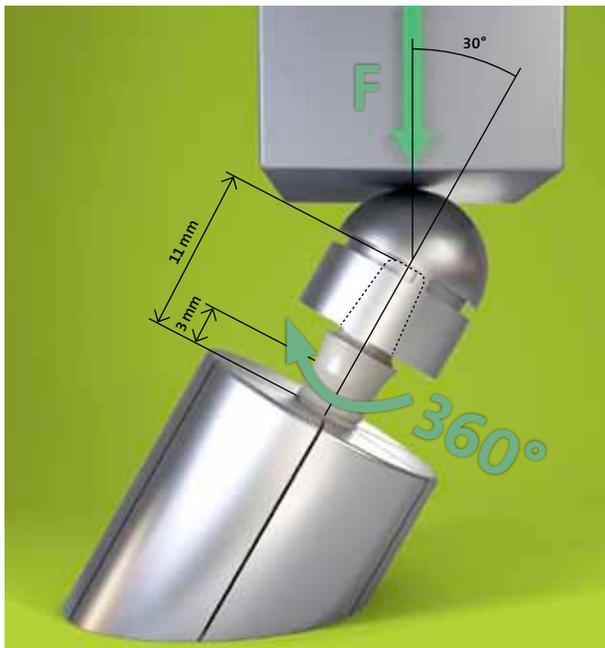
Fig. 1: Test setup according to ISO 14 801
